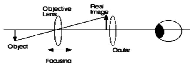
**Fig. 2** Focusing of light by an objective lens results in a magnified real image of the object which can be imaged by the ocular.
