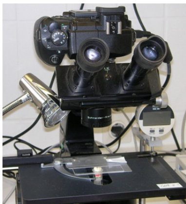
Fig. 1 Digital reflex camera coupled to the orthostat for photography.
