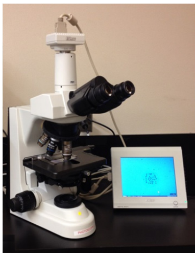
Fig. 3 Nikon Eclipse 50i microscope with Nikon DS-Fi Digital Sight camera and monitor.
