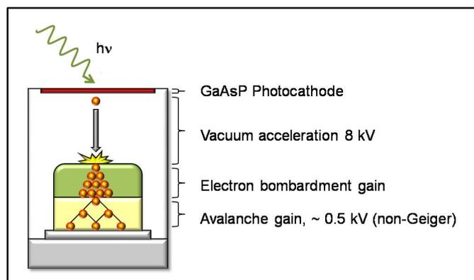
**Fig. 3** Schematic drawing of a hybrid detector
