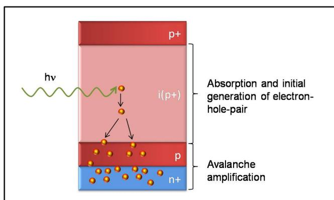
**Fig. 2** Upon absorption of photons in an intrinsic (i-) layer, an electron-hole pair is generated. The avalanche is caused in a multiplication zone (pn+) by impact ionization through the arriving electrons.
