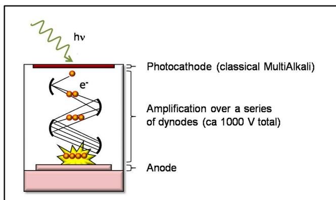
**Fig. 1** Schematic drawing of a photomultiplier tube. The photon energy is converted into accelerated electrons at the photocathode. Subsequently following dynodes multiply the initial photoelectron by secondary emission. The multiplication at each step depends on the potential difference between the dynodes, which is  $1/n$  of the total high voltage applied when the tube contains  $n$  dynodes.
