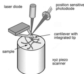
**Figure 1:** Principle of AFM. The sample is positioned by a xyz piezo scanner. The deflection is detected by a laser beam focused on to the end of the cantilever and reflected onto a position sensitive detector. (Edited from [13])
