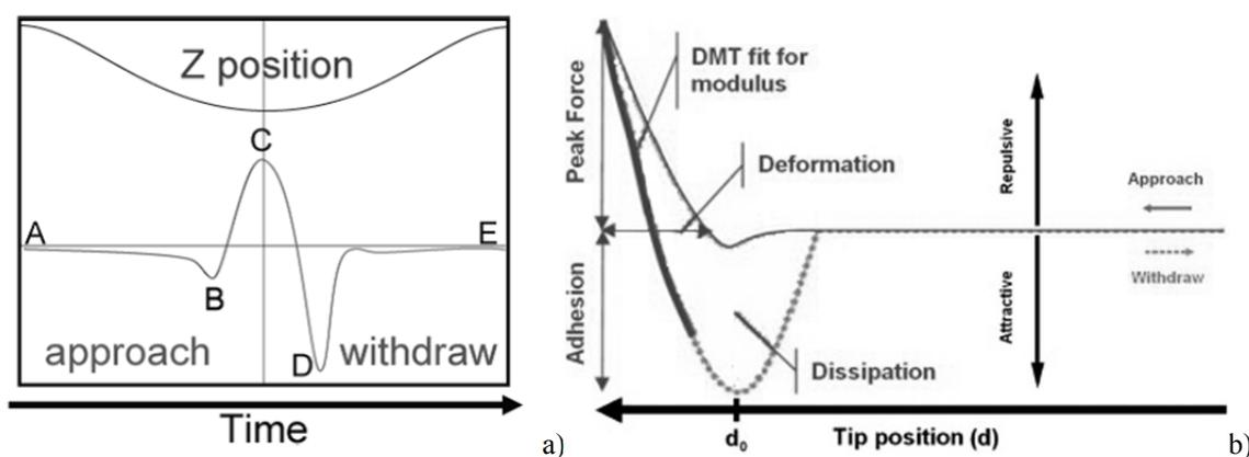
**Figure 2:** Force curves for a single cycle of peak force tapping a) a force and the Z position as a function of time b) plot of the force vs. z-displacement and how the different material properties are extracted (Edited from [23]).
