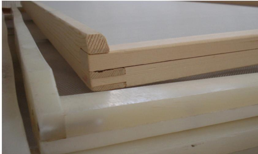
**Fig. 1** Wooden and plastic trays for pasta drying
