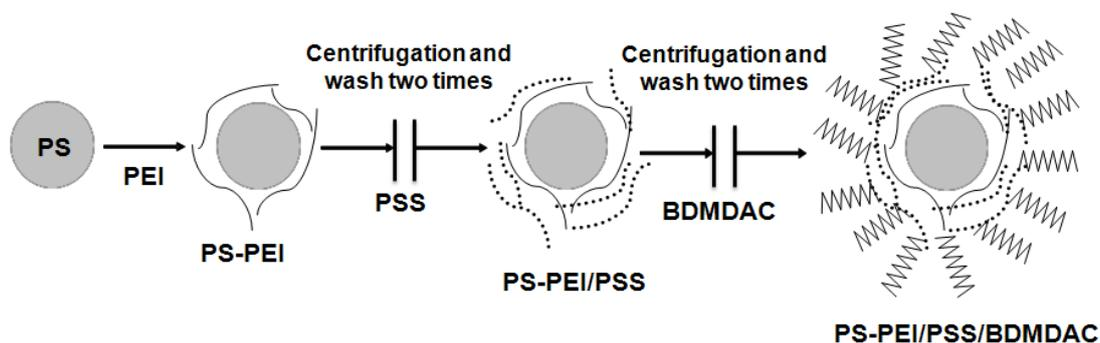
**Figure 4** – Schematic representation of the particles production process. (PEI-polyethyleneimine, PSS- sodium polystyrene sulfonate and BDMDAC- benzildimethyldodecyl ammonium chloride).
