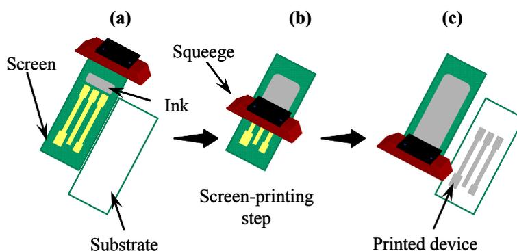
Fig. 3 Screen-printed device fabrication process scheme: (a) Ink poured; (b) Squeegee traversing; (c) Ink deposited on the substrate surface
