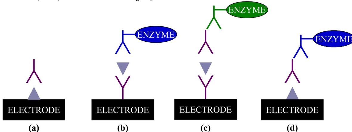
**Fig. 4** Schematic diagram of the different assay formats used in disposable electrochemical immunosensors: (a) Direct assay; (b) Direct sandwich assay; (c) Indirect sandwich assay; (d) Indirect assay
