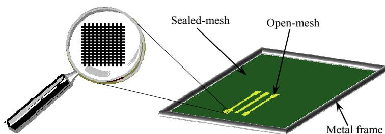
Fig. 2 Scheme of a screen
