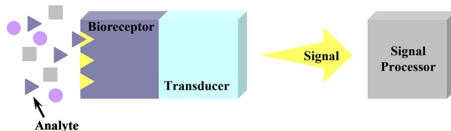
Fig. 1 Scheme of a biosensor
