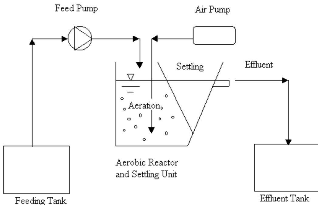
**Fig. 1** A schematic diagram of the activated sludge bioreactor used in experimental studies.
