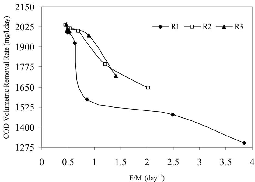
**Fig. 3** The effect of F/M ratios on COD volumetric removal rates in the control and test reactors.
