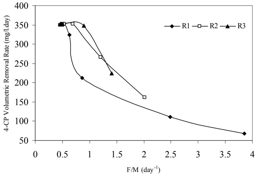
**Fig. 2** The effect of F/M ratios on 4-CP volumetric removal rates in the control and test reactors.
