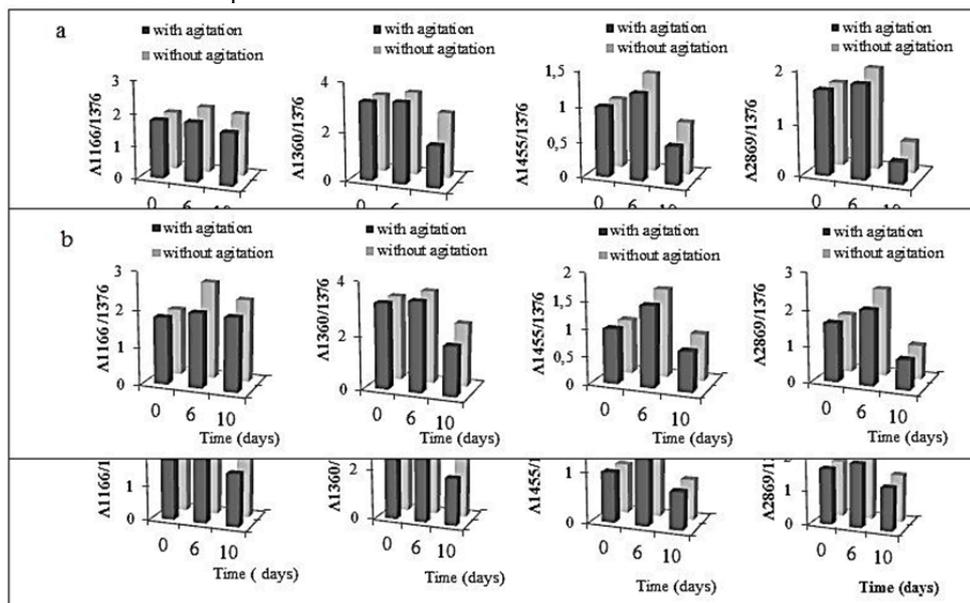
**Fig. 2** Variation of absorbance's ratios as a function of time of contact with: a) Sunflower oil at 40°C; b) Sunflower oil at 20°C; c) n-octane at 40°C
