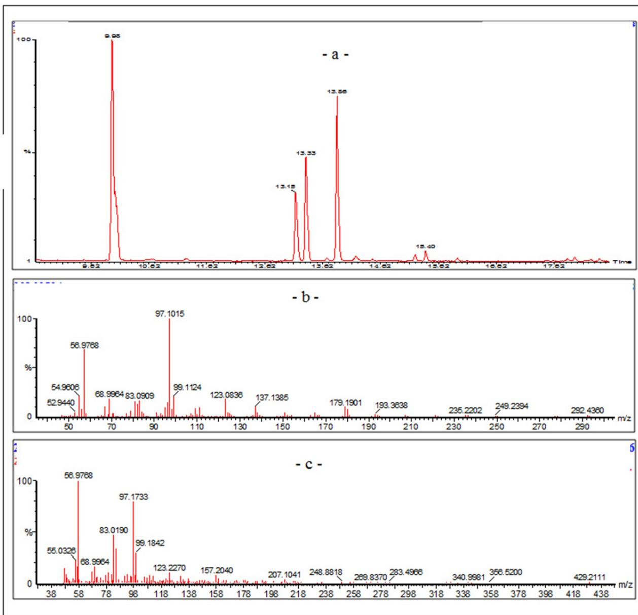
**Fig. 3** a) Chromatogram of the sample in contact with the sunflower oil for 10 days without agitation at 20°C; b) Fragmentation of the peak retention time of 9.98min; c) Fragmentation of the peak retention time of 13.86min.
