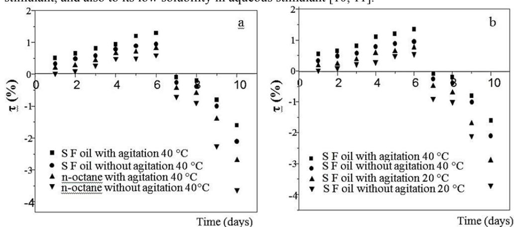
**Fig. 1** Evolution of the rate of mass variation versus time of contact in the case of sunflower oil and n-octane with and without agitation at 20 and 40 °C. **a)** highlight the influence of the agitation and the nature of food simulant; **b)** highlight the influence of temperature
