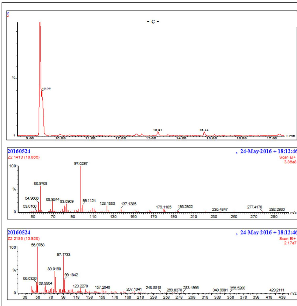
**Fig. 4** a) Chromatogram of the sample in contact with the sunflower oil for 10 days without agitation at 40 °C; b) Fragmentation of the peak time retention of 10.01min; c) Fragmentation of the peak time retention of 13.91min.
